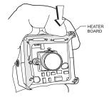
2. If the heater is installed, plug the heater connector from the camera into the mating connector inside the base. Plug the video connector from the camera into the mating connector inside the base.
